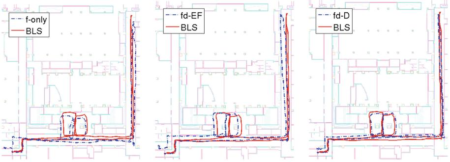
**Fig. 4.** Estimated trajectories for three of the four resource-allocation schemes considered against the BLS groundtruth overlaid on the building’s blueprint.
